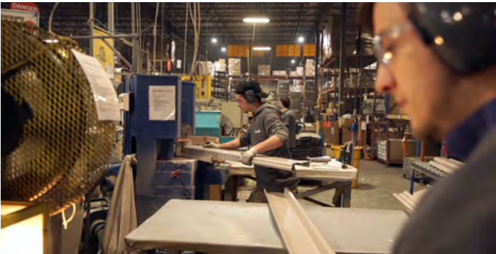
Perforation des margelles. Perforating the top seats.
